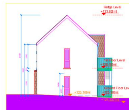
Block D - East Elevation
