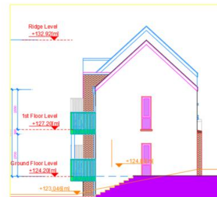
Block D - West Elevation
